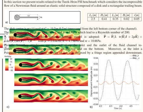
The amplitude of the last period of oscillation is in the range of 0.03 m for the vertical displacement and of 0.0025 m for the horizontal displacement; the frequency of the *y*-displacement is about  $6 s^{-1}$ , and the frequency for the *x*-displacement is about  $12 s^{-1}$ . All values are in good agreement with the original benchmark results [3]. The vorticity in the fluid ranges from  $-30 s^{-1}$  to  $30 s^{-1}$ .
